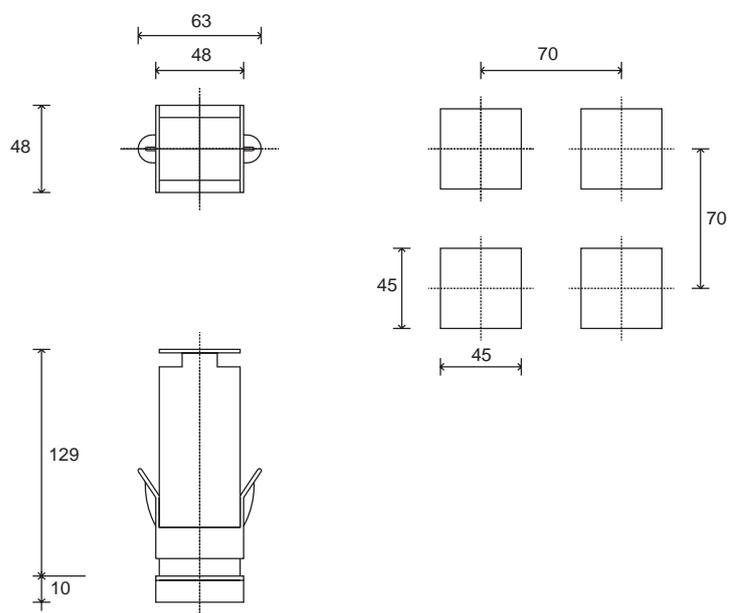
Dimensions: 48x48mm (1/16DIN), profondeur 129mm
