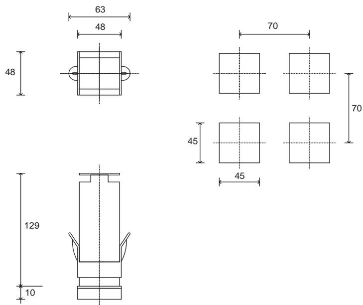
Dimensions: 48x48mm (1/16DIN), profondeur 129mm
